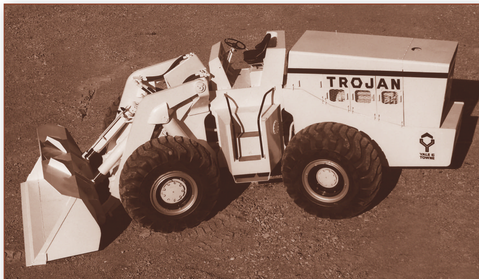
Trojan 8000 measured 32 feet 7 inches from rear to bucket tip, 12 feet 2 inches from ground to top of cab, and just under 12 feet in overall width.
