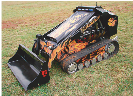
The Super Witch VI is remote controlled and has a shut-down switch on the control panel. At every performance, a second remote, in the hands of an observer with a good view of the area, also has a shutdown switch.
