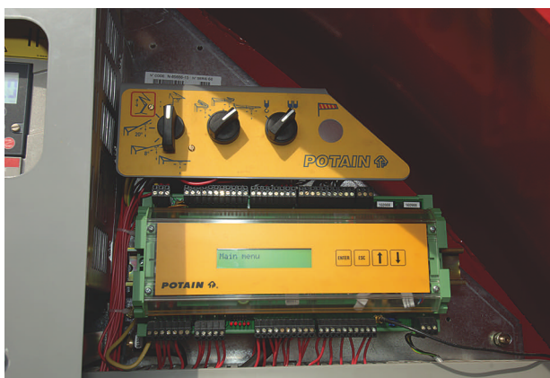
The remote controller (left) provides a visual display of the crane's operating parameters. The switch panel in the machine's right-side cabinet (right) is used to select set-up modes and to set operating conditions.
