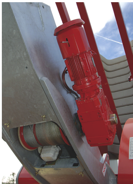
The electric motors for the Igo 50's hoist, trolley, swing and hydraulic pump are accessible from ground level — as are the winches for hoist and trolley. The drum for the trolley line, shown here, is positioned in the base of the mast.
