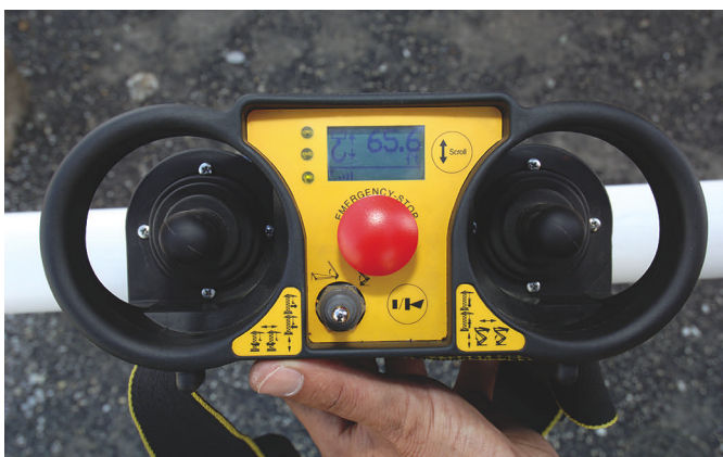
The remote controller (left) provides a visual display of the crane's operating parameters. The switch panel in the machine's right-side cabinet (right) is used to select set-up modes and to set operating conditions.
