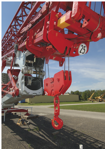
The electric motors for the Igo 50's hoist, trolley, swing and hydraulic pump are accessible from ground level — as are the winches for hoist and trolley. The drum for the trolley line, shown here, is positioned in the base of the mast.
